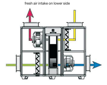
CompAir RW with 4 top connections (V) - 3 sizes, airflows up to 4700 m³/h
