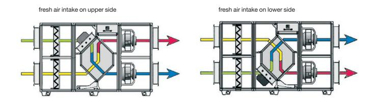
CompAir CF with 2 side and 2 top connections (HV)\* - 7 sizes up to 10 700 m³/h
