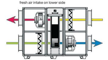
CompAir RV with 2 side and 2 top connections (HV)\* - 6 sizes, airflows up to 10 700 m³/h
